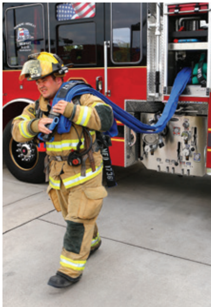
Lower crosslay height for easier hose removal
