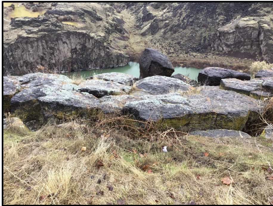
Photograph 4. Site conditions, looking north at the canyon rim, north of the project site. Discontinuity spacing in photograph is approximately 24 inches.
