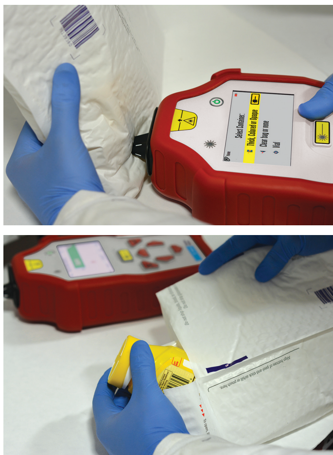
Figure 1. The Agilent Resolve system has the unique capability to scan through multiple opaque layers of packaging without any prior knowledge of the sample. This example consists of pills contained within opaque plastic and mailer bag.
