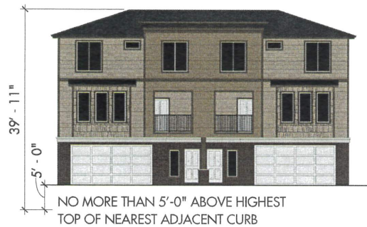
3 CE-105L 1/8" = 1'-0" BUILDING R - FRONT ELEVATION
