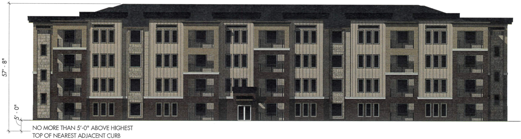
1 BUILDING K - FRONT & BACK ELEVATION 1/8" = 1'-0"
