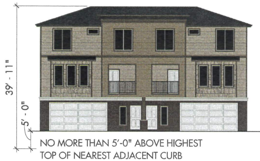
3 CE-105L 1/8" = 1'-0" BUILDING R - FRONT ELEVATION
