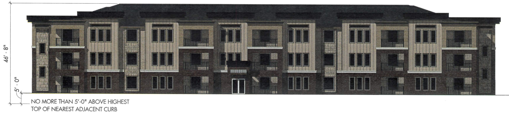
1 BUILDING K - FRONT & BACK ELEVATION 1/8" = 1'-0"
